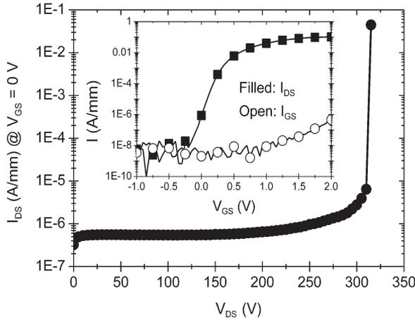
Fig. 3. Three-terminal OFF-state breakdown characteristic measured at  $V_{GS} = 0$  V with  $V_{DS}$  step of 5 V. Inset shows  $I_{DS}$  and  $I_{GS}$  semilog transfer characteristics at  $V_{DS} = 10$  V. The ON/OFF ratio at  $V_{GS} = 2$  V/0 V is  $10^5$ . Gate-to-drain spacing is  $3 \mu\text{m}$ .
