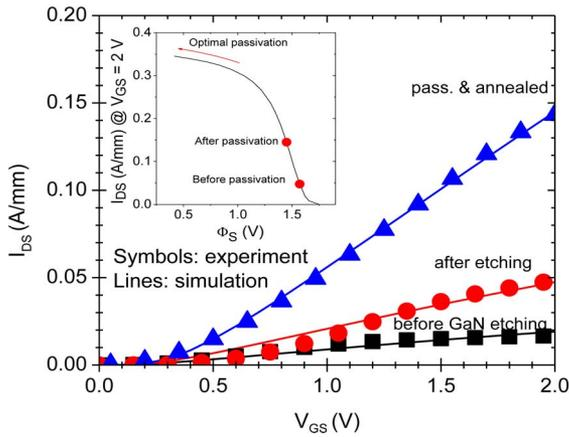
Fig. 4. Experimental and calculated transfer characteristics of the GaN/InAlN/AlN/GaN HEMT at various stages of the processing. Inset shows the calculated dependence of  $I_{DSmax}$  on  $\Phi_S$  (InAlN). In the inset, points correspond to the experimental results, and the arrow indicates the range of the surface potential for the anticipated optimal passivation.
