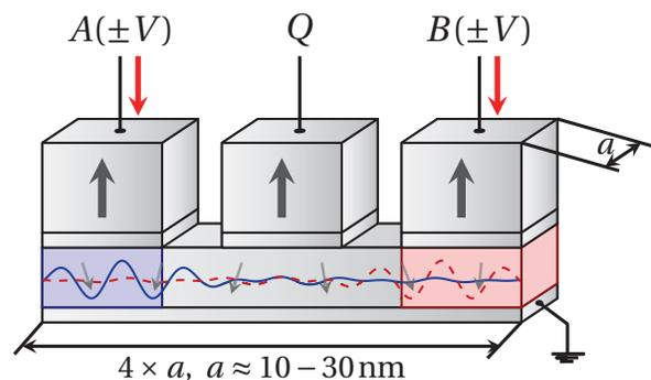
Fig. 1. Non-volatile magnetic flip flop exhibiting a shared free layer storing the information via magnetization orientation, two stacks  $A, B$  for input and one stack  $Q$  for output. The current (voltage) polarities and the magnetization orientation of the free layer are mapped to logic "0" and "1".
