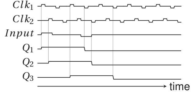
Fig. 5. Example signal sequence illustrating how information is written into the first flop  $Q_1$  ( $Input$  and  $Clk_1$  exhibit same polarities), then passed to the second flip flop  $Q_2$  ( $Q_1$  and  $Clk_2$  same polarity) and from there to the third flip flop  $Q_3$  ( $Q_2$  and  $Clk_1$ ).
