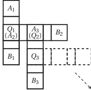
Fig. 3. Top view of an alternative cross topology for a two level shift register. Odd (even) flip flops are in the top (bottom) layer.
