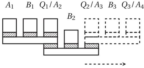
Fig. 2. Side view of a shift register topology enabling information transport via spin transfer torque. Either the first level ( $A_1, B_1, Q_2/A_3, B_3, \dots$ , first clock signal  $Clk_1$ ) is powered or the second level is active ( $Q_1/A_2, B_2, \dots$ , second clock  $Clk_2$ ) passing the information stored in the shared free layers between the subsequent flip flops.
