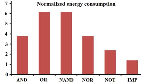
Fig. 4. The normalized energy consumption of IMP-based implementations of basic Boolean logic operations. The energy is normalized in the amount of that required for antiparallel-to-parallel MTJ switching ( $E_{\text{AP}\rightarrow\text{P}}$ ).
