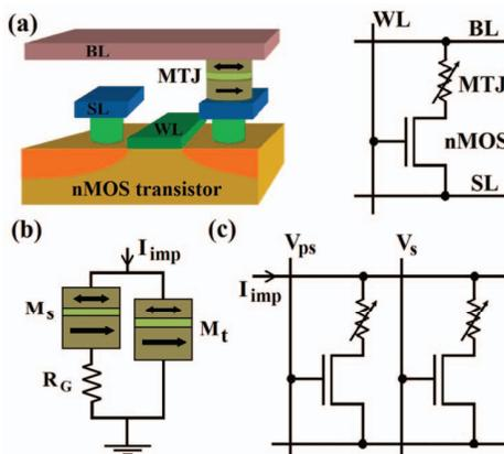
Fig. 1. (a) Structure and equivalent circuit of 1T/1MTJ cell. (b) Current-controlled MTJ-based IMP logic gate [3] including source ( $M_s$ ), target ( $M_t$ ) MTJs. (c) Proposed MRAM-based IMP logic gate. By applying  $V_{ps}$  ( $V_s$ ) to a word line the source (target) MTJ is selected.
