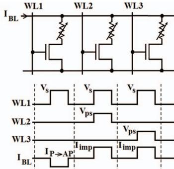
Fig. 3. Proposed MRAM-based array for IMP logic implementation and required circuit signals for performing universal NOR operation in three steps.
