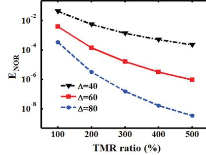
Fig. 5. The error probability for the universal NOR operation implemented based on the proposed MRAM logic array as a function of the TMR ratio plotted for different values of  $\Delta$  and optimized circuit parameters.
