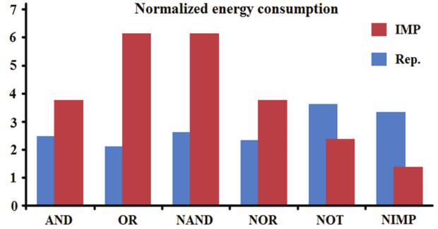
Fig. 6. Normalized energy consumption of the Boolean logic operations shown in Fig. 5. The energy is normalized by the amount of energy required for high-to-low MTJ resistance switching ( $\sim 18$  pJ for  $t = 50$  ns, based on physical devices characterized in [11]).
