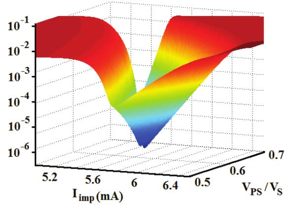
Fig. 3. Circuit parameters ( $I_{\text{imp}}$ ,  $V_s$ , and  $V_{\text{ps}}$ ) optimization for minimum implication gate error probability with MTJs characterized by  $R_P = 1.8\text{k}\Omega$ ,  $\text{TMR} = 3$ , and  $\Delta = 70$ .
