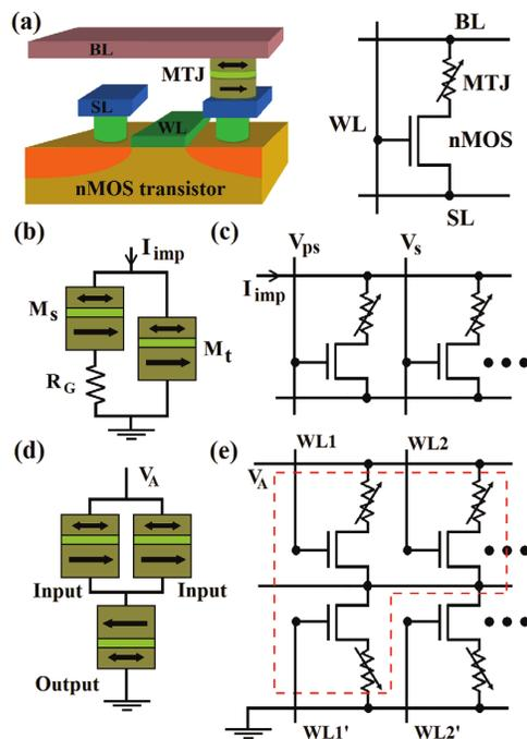
Fig. 1. (a) Structure and equivalent circuit of 1T/1MTJ cell. MTJ-based implication (b) [5] and reprogrammable (d) [6] logic gates. 1T/1MTJ-based realization of implication (c) and reprogrammable (e) logic gates.
