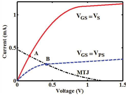
Fig. 2. Bias points of the access transistor in a 1T/1MTJ cell for the selecting (point A) and pre-selecting (point B) voltages applied to the word line of the cell.
