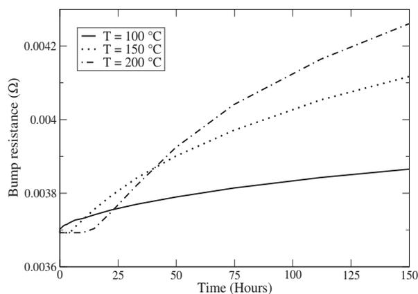
Fig. 7. Initial phase of solder bump resistance growth for three different temperatures.
