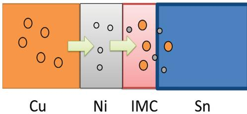
Fig. 3. EM of Cu and Ni atoms into Sn bump and the forming of IMC.
