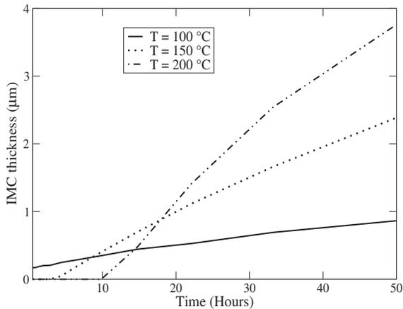
Fig. 8. Growth of IMC thickness in time. Fast migration of Cu and Ni at 150°C and 200°C prevents IMC emergence for several hours of stressing.
