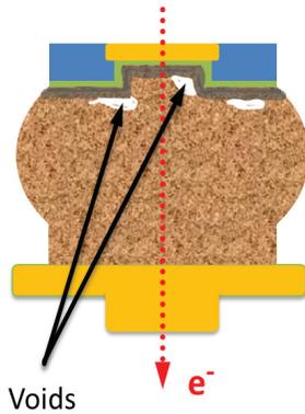
Fig. 1. EM failure is caused by voids which are formed between Ni under bump metallization (UBM) and Sn solder bump.
