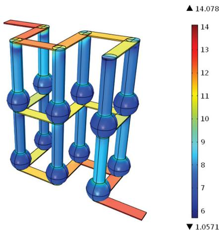
Fig. 4. Multilevel interconnect for 3D integration. Presented is the current density distribution on the logarithmic scale ( $\times 10^3 \text{ A/cm}^3$ ). Wafers are removed from the picture. The copper TSV length is  $100 \mu\text{m}$  and the diameter chosen  $25 \mu\text{m}$ . The UBM thickness is  $2.5 \mu\text{m}$  and the bump diameter is  $40 \mu\text{m}$ . Due to the chosen geometry the lowest calculated current density is inside the bumps ( $2.66 \cdot 10^3 \text{ A/cm}^2$ ).
