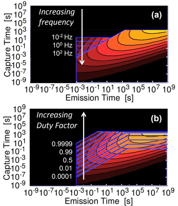
Fig. 6: Analogously to Fig. 5a, the CET map of Fig. 4b overlaid with an occupancy map allows representing stress at (a) different frequencies and (b) duty factors. (a) A weak frequency  $f$  dependence is expected at low frequencies [9]. At higher frequencies the occupancy tends toward beveled rectangle delimited by  $t_{stress}$  and  $t_{relax}$ . (b) The beveled-rectangle region increases with increasing Duty Factor ( $f = 1$  kHz).
