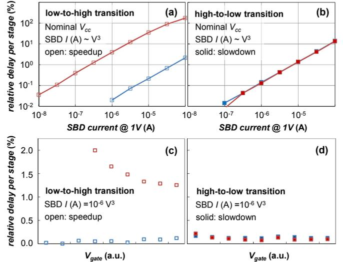
Fig. 14: (a-b) Circuit simulations show that a non-ohmic SBD (red/blue BD location definition cf. Fig. 12) of the expected magnitude  $< 1 \mu\text{A}$  @ 1V will have a limited impact on circuit delay (in fact, speedup for low-to-high delay is expected (a)). (c-d) Although increased  $V_{gate}$  will accelerate BD, the impact of SBD on the delay will *not* be higher at higher  $V_{gate}$ .
