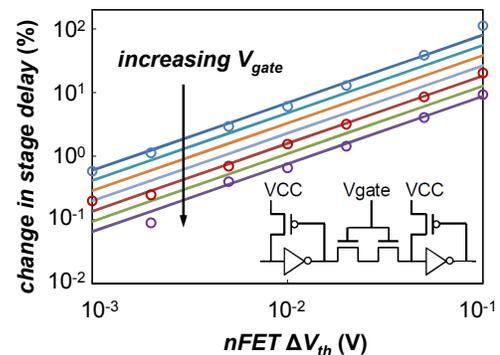
Fig. 1: SPICE-simulated change in average stage delay (symbols; circuit in inset) as a function of the nFET threshold voltage shift  $\Delta V_{th}$ . The dependence is parameterized (lines). Note that the  $\Delta V_{th}$  impact on stage delay increases exponentially as  $V_{gate}$  is lowered toward  $V_{CC}$ , documenting the vulnerability of this topology toward PBTI.
