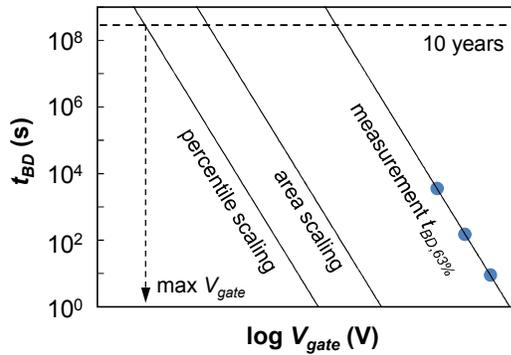
Fig. 15: HBD projection determines the maximum  $V_{gate}$  (see also Fig. 11c). Analytical technique to reduce across-wafer variability [19] and the total gate area of all sub-circuitry exposed to higher  $V_{gate}$  are used.
