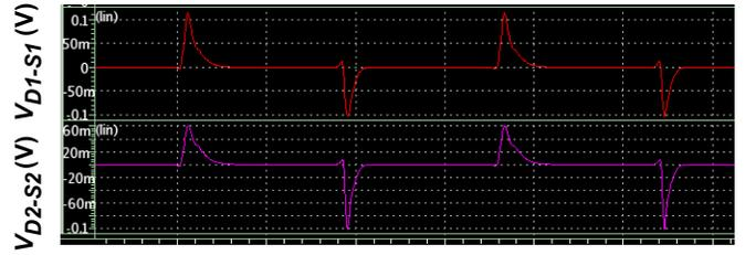
Fig. 13: Circuit simulations show the serially connected nFETs will not be subjected to hot carrier degradation conditions (max  $V_{d-s}$  bias  $\sim 0.1$  V, node definitions cf. Fig. 12).
