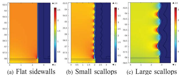
Fig. 7. Current density distribution (MA/cm<sup>2</sup>) in the three filled copper TSVs when a 1A current is applied through the top of the structure.
