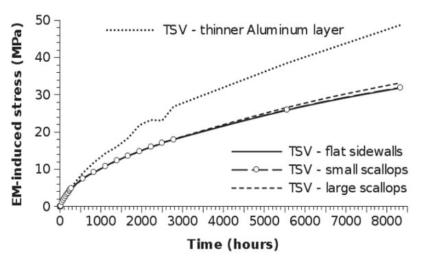
Fig. 15. Maximum EM-induced stress (MPa) through the aluminum layer in the open tungsten TSVs, while operating with a 1A current applied through the structure.
