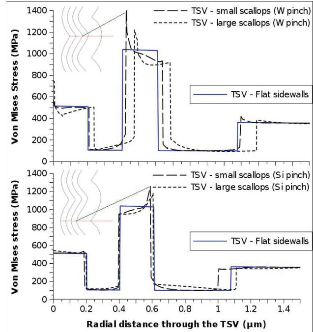
Fig. 12. Von Mises stress through the vertical middle of the open tungsten TSVs assuming a drop from a stress-free temperature of 320°C to 20°C.
