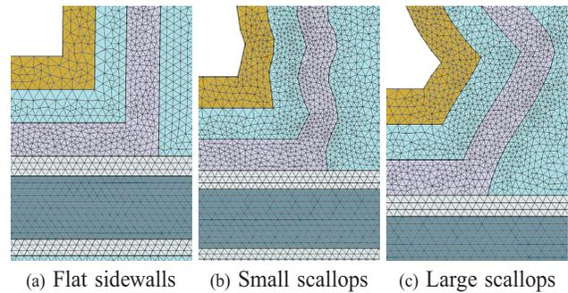
Fig. 4. Mesh at the bottom of the three filled copper TSVs. The image is an enhanced section from Fig. 3 where the oxide, tungsten, titanium nitride, aluminum, and silicon nitride layers are visible.
