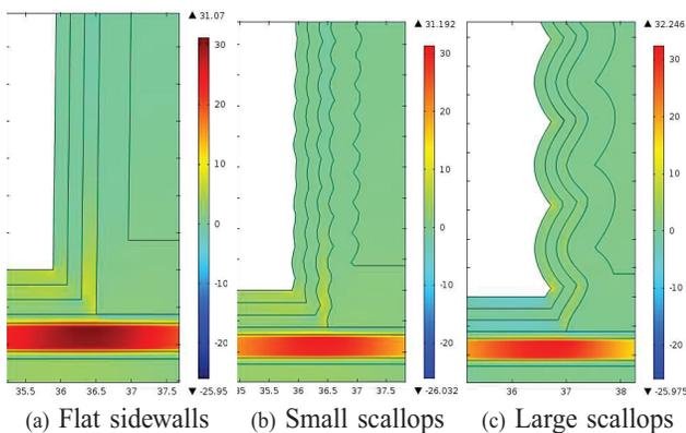
Fig. 14. Electromigration-induced stress (MPa) in the aluminum layer of the three open tungsten TSVs when a 1A current is applied through the structure for one year.
