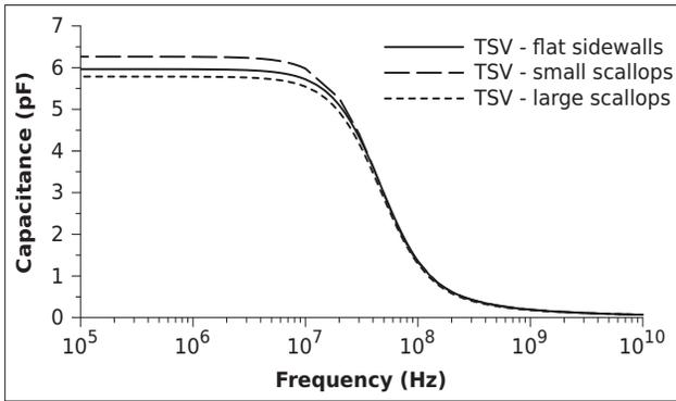
Fig. 10. Frequency-dependent capacitance (pF) for the three open tungsten TSVs shown in Fig. 3.
