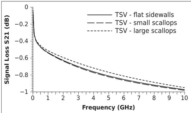
Fig. 11. Frequency dependence on the signal loss S21 (dB) for the three open tungsten TSVs. A higher loss is noted at high frequencies for the large-scalloped structure.
