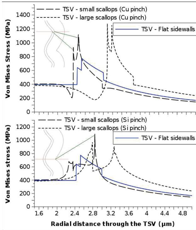
Fig. 6. Von Mises stress through the vertical middle of the filled copper TSVs assuming a drop from a stress-free temperature of 320°C to 20°C.
