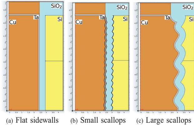
Fig. 1. Materials at the top of the three filled copper TSVs. The backside (bottom) of the structure is also connected to a copper layer, through a tantalum liner.
