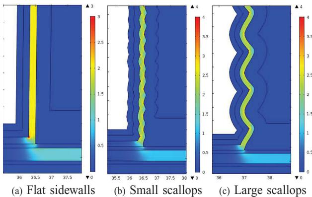
Fig. 13. Current density distribution ( $\text{MA}/\text{cm}^2$ ) in the aluminum layer of the three open tungsten TSVs when a 1A current is applied through the structure.
