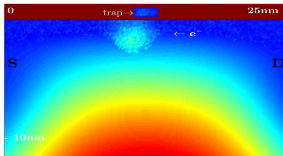
Fig. 6. The electron state moves in a MOSFET potential and charges the trap into the oxide by tunneling trough the thin barrier with the channel.
