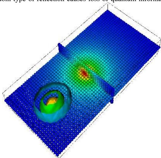
Fig. 3. Three-dimensional electron density in proximity of a Phosphorus dopant. A channel dopant may block an area larger than its geometric characteristics due to the nonlocality of the quantum interaction.
