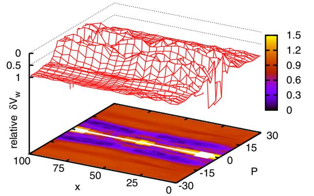
Fig. 5. The relative absolute difference of the probability distributions (normalized WPs) calculated with and without the application of a smoothing Tukey window ( $\alpha = 0.2$ ), using Profile 2 (blue) in Fig. 1. A coherence length of  $\mathbf{L} = \mathbf{L}_{dev}$  is used, along with boundary approach i) discussed in the text.
