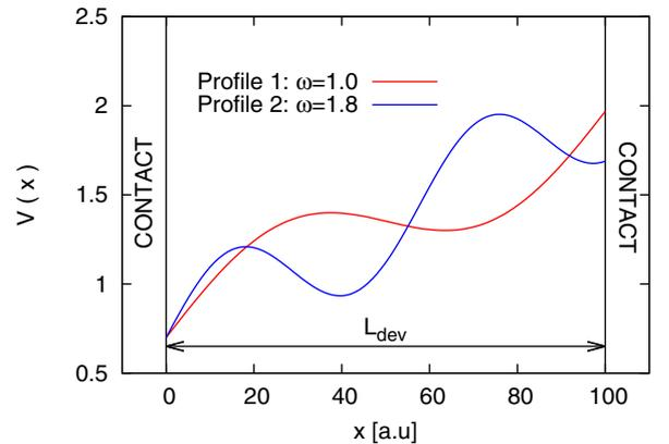
Fig. 1. Two analytic potential profiles, of the form (3), with known spectral content ( $\omega$ ) and a bias between the left and the right contacts of 1.3 V.
