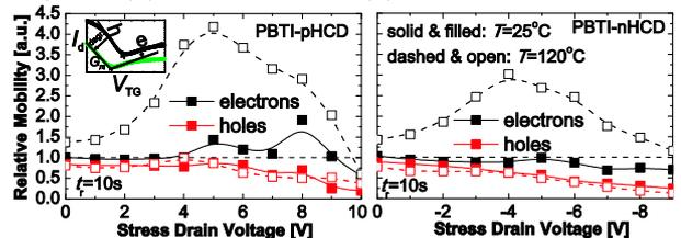
Fig.3: Relative mobility vs.  $V_d$  for PBTI-pHCD and PBTI-nHCD. The inset shows the mobility estimation scheme.
