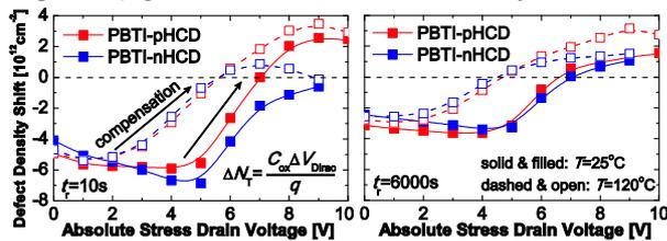
Fig.2: Defect density shift vs.  $V_d$  measured at two relaxation time points and different  $T$ .
