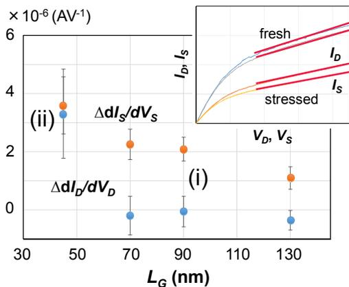
Fig. 9: Change in  $dI_d/dV_d$  ( $dI_d/dV_s$ ) slope after CHC stress (inset) allows visualizing CHC degradation (i) longitudinally localized in longer nFinFETs and (ii) spanning the entire channel in shorter devices. BTI degradation is symmetric at all  $L_G$ 's (not shown).
