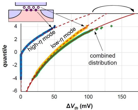
Fig 13: Bimodal defect-centric distribution  $\Delta V_{th}$  corresponding to CHC stress: Monte Carlo and analytic fit [24]. The high- $\sigma$  tail of the full distribution is controlled by defects at the substrate (high  $\eta$ ; inset: solid symbols).
