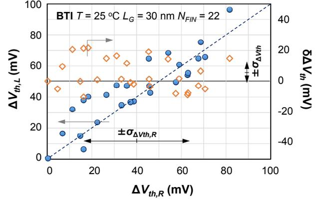
Fig. 2: Illustration of an extreme case of across-wafer variability affecting time-dependent variability due to BTI stress. Note the correlation  $\Delta V_{th,L}$  and  $\Delta V_{th,R}$  in individual MPs due to the systematic variability (solid circles) and the reduction of variance  $\sigma_{\Delta V_{th}}^2$  when Eq. 3 is used on the MP degradation difference  $\delta \Delta V_{th}$  (Eq. 2, open diamonds).
