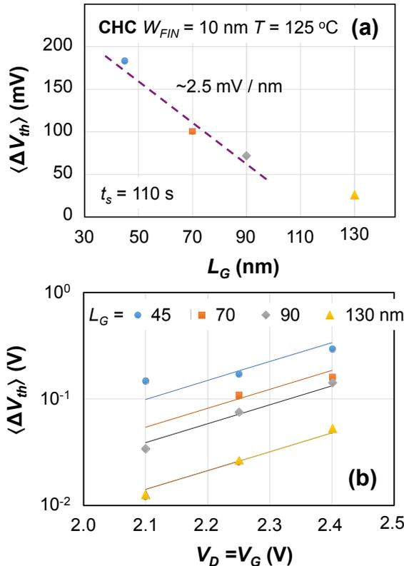
Fig. 5: Sensitivity of CHC to (a)  $L_G$  and (b) bias.
