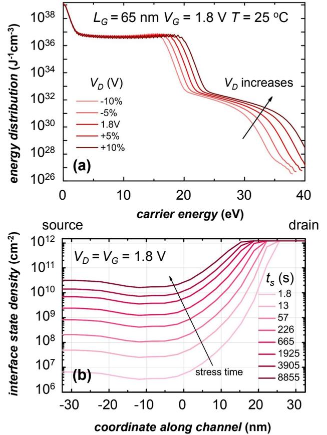
Fig. 6: CHC simulation in a planar device. (a) CHC energy distribution at drain (cf. Fig 4a), responsible for trap generation and charging, is sensitive to drain bias. (b) Increase in CHC degradation along the channel. Note the most damaged region extending  $\sim 20$  nm from the drain.
