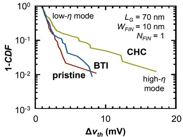
Fig. 12: An example of single-trapping-event  $\Delta v_{th}$  distributions obtained from TDDS measurements [15] show distinct increased defect density close to channel/oxide interface (high- $\eta$  mode; cf. Fig. 4d) after CHC stress. Low- $\eta$  mode corresponds to charged defects deeper in the gate oxide.
