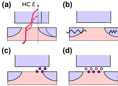
Fig. 4: Sources of increased CHC variability: (a) Channel length/LER and schematic CHC energy distribution, (b) series resistance, (c) longitudinally and (d) vertically non-uniform trapping.
