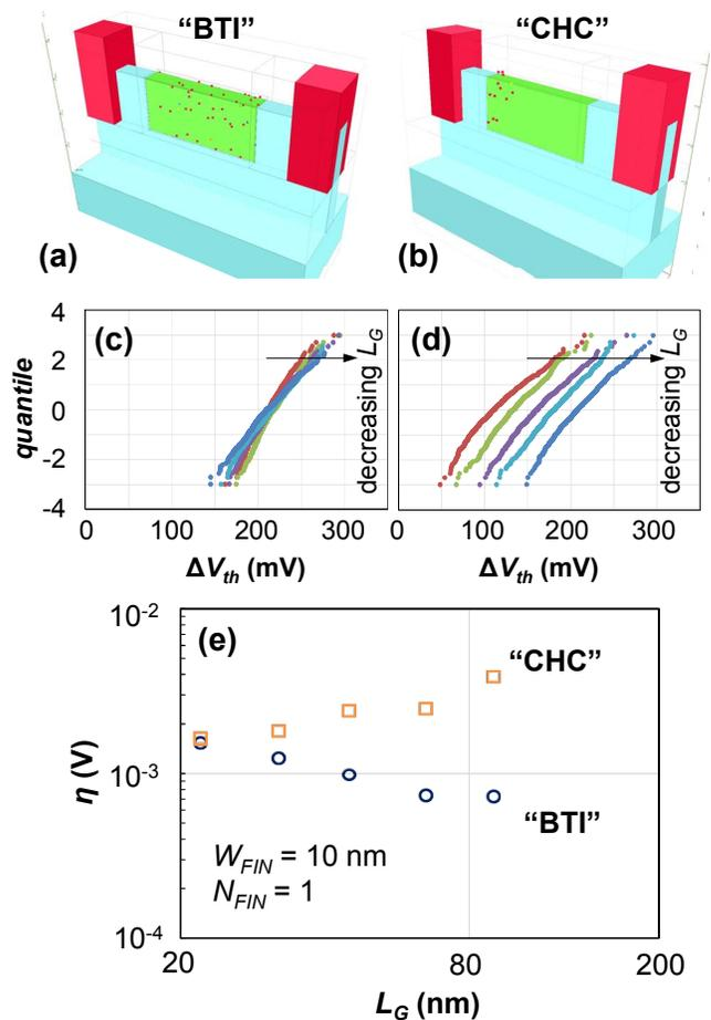
Fig. 10: "Atomistic" TCAD simulation [19] of (a) uniform ("BTI") and (b) localized (20 nm from the drain, "CHC") trapped charge (with constant density) in *synthetic* nFinFETs results in distributions (c) and (d), respectively, as a function of  $L_G$ . (a) Values of  $\eta$  calculated through Eq. 1 qualitatively well reproduce measured dependence (open symbols) in Fig. 8.
