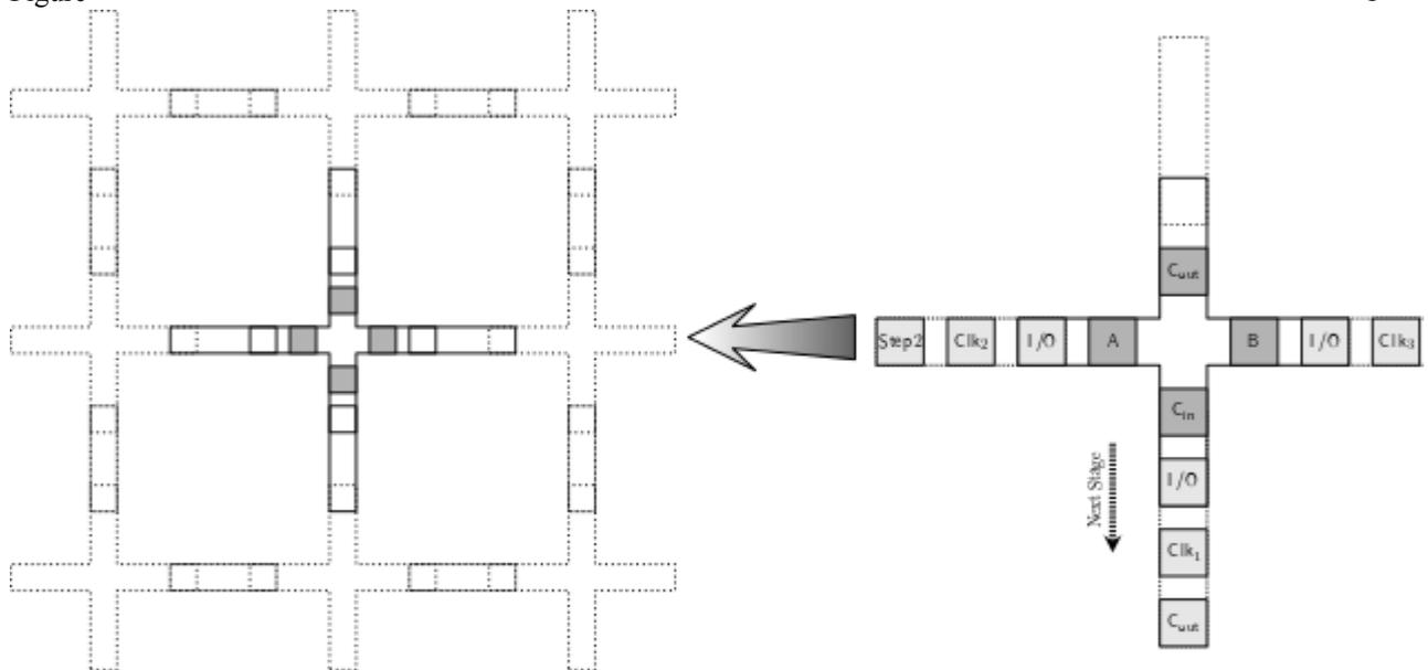
Figure 1: Illustration of the proposed buffered magnetic logic gate gri and an example for a 1 bit full adder realized with a single majority g and three flip flops as buffers.
