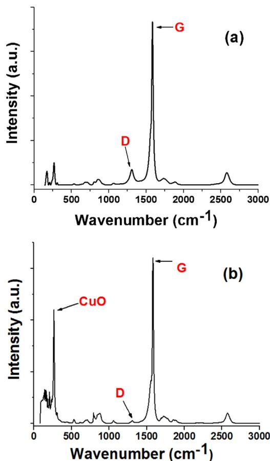
**Fig. 3.** Raman spectra of the (a) SWCNTs after acid treatment and (b) SWCNTs after decoration with Cu NPs.
