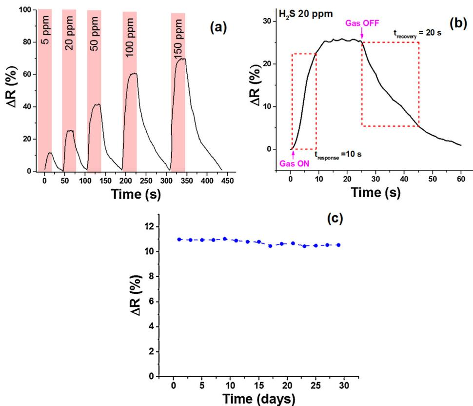
**Fig. 4.** (a) Sensor response to various  $H_2S$  gas concentrations at room temperature. (b) Enlarged response curve of the sensor under exposing to 20 ppm  $H_2S$  (c) Long-term evaluation of the sensor's response to 5 ppm  $H_2S$  gas at room temperature.
