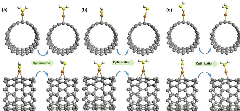
**Fig. 10.** The optimized structures for a single H<sub>2</sub>S molecule adsorbed on a SWCNT with three possible configurations: (a) S atom is the nearest atom to Cu-SWCNT, (b) S atom is the nearest atom to Cu-SWCNT [with 90° rotation of (a)], and (c) the H atom is the nearest atom to Cu-SWCNT.
