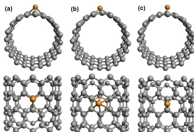
**Fig. 8.** Three possible configurations Cu-SWCNT: (a) directly above a C atom, (b) at the center of hexagon and (c) at the center of a C–C bond (bridge site).
