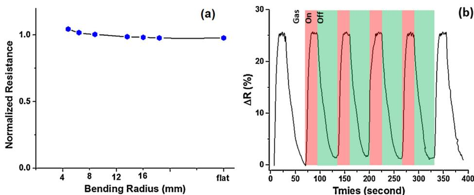
**Fig. 6.** (a) normalized resistance of the Cu-SWCNTs-based flexible devices as a function of the bending radius and (b) the sensor response upon exposure to 20 ppm  $H_2S$  gas and a bending radius of 7.8 mm.
