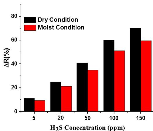
**Fig. 7.** Final response of the Cu-SWCNTs based flexible sensor under 40% relative humid and dry environment at room temperature.
