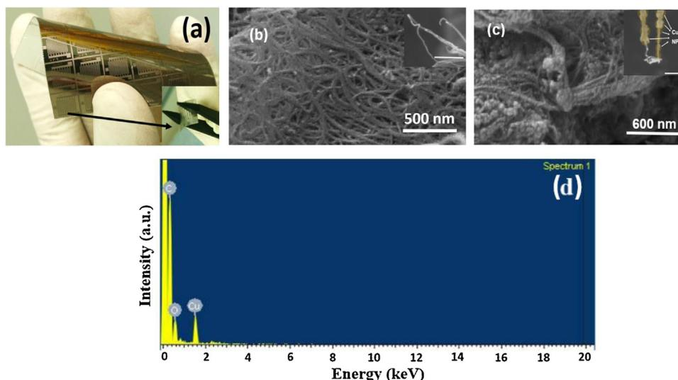
**Fig. 2.** (a) Optical image of the fabricated devices on the flexible substrate. The inset depicts a single device. SEM images of (b) bare SWCNTs after acid treatment (the inset figure scale bar is 600 nm) and (c) after decoration with Cu NPs which shows successful decoration of sidewalls with NP clusters (the inset figure scale bar is 500 nm). (d) EDS analysis of Cu-SWCNTs sensitive material.
