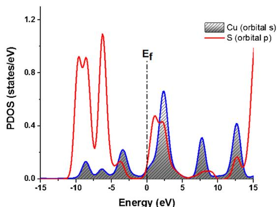
Fig. 13. The PDOS of Cu atom (3p-orbital) overlapped with S atom (4s-orbital) in the H<sub>2</sub>S/Cu-SWCNT system. The Fermi level is shifted to the zero point.
