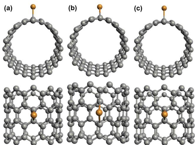
**Fig. 9.** Optimized configurations of Cu-SWCNT. The forces on each atom are being smaller than 0.05 eV/Å and the cutoff energy is 150 Ry.
