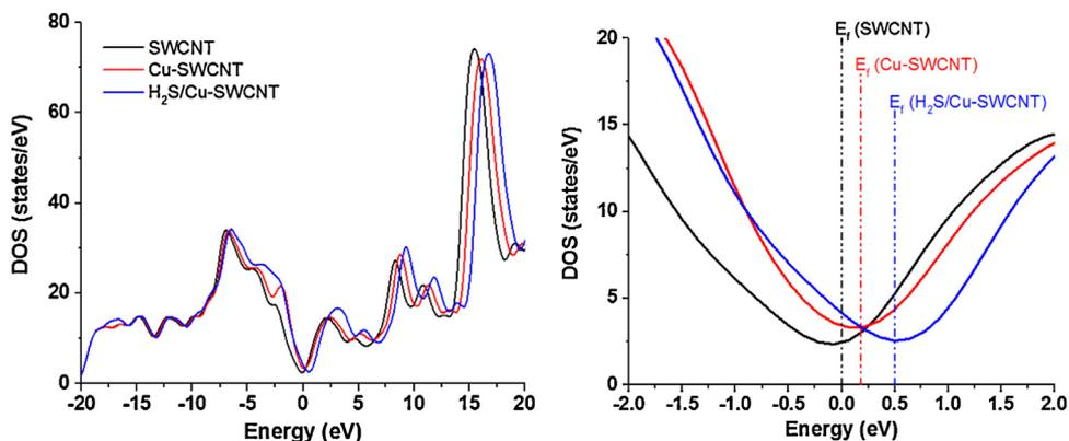
**Fig. 11.** The DOS of SWCNT, Cu-SWCNT, and H<sub>2</sub>S/Cu-SWCNT.
