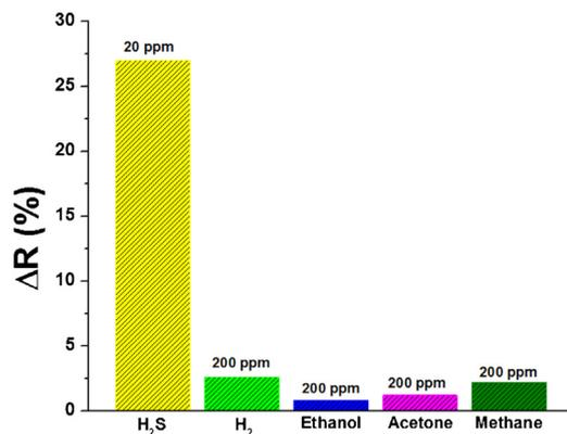
**Fig. 5.** The selectivity of the fabricated sensors to various gases. The  $H_2S$  concentration is kept at 20 ppm while the concentrations of other interfering gases are fixed at 200 ppm.
