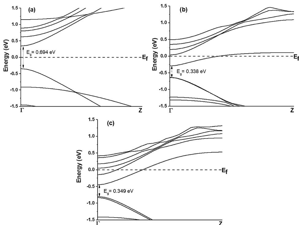
Fig. 12. The electronic band structure of the (a) pristine (10,0) SWCNT, (b) Cu-SWCNT and (c) H<sub>2</sub>S/Cu-SWCNT system. Fermi energy is shifted to the zero point.
