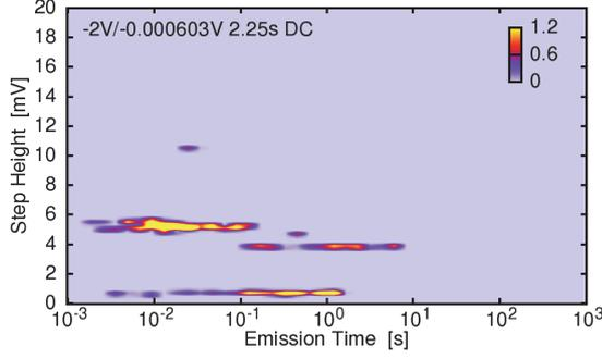
Fig. 5: Time-Dependent Defect Spectroscopy (TDDS) spectrum of three traps in a single FinFET device. The distribution of emission times and impacts on the FinFET  $V_{th}$  (“step height”) is apparent. The TDDS technique was developed specifically within the defect-centric approach [16].
