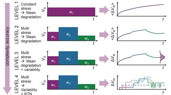
Fig. 14. Complexity/accuracy levels of incorporating device aging (specifically here, the threshold voltage shift) in circuit simulations. The full workload on each device can be *approximated* by a series of phases  $w_i$  with duration  $t$ , voltage  $V_i$ , duty factor  $DF$ , frequency  $f$ , and temperature  $T$ . (In reality the number of workload phases is typically very large.)
