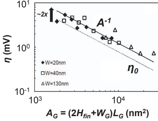
Fig. 9: The average impact per trap  $\eta$  as  $A_G^{-1}$  in pFinFETs (high-k/MG,  $t_{inv} \approx 1.7\text{nm}$ ) with varying fin width  $W_G$  and gate length  $L_G$  (fin height  $H_{fin}$  is fixed). Each point is extracted from a distribution such as those in in Fig. 8. The value of  $\eta$  is  $\sim 2\times$  higher than the expected  $\Delta V_{th}$  for a single charge from a charge sheet approximation  $\eta_0 = q/C_{ox}$  [29].
