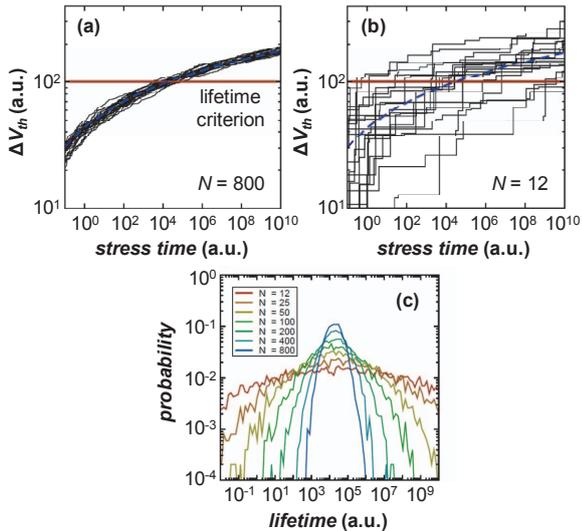
Fig. 2: (a) The random properties of many defects  $N_T$  in large devices average out, resulting in a well-defined lifetime while (b) the stochastic nature of a handful of defects in deeply-scaled devices becomes apparent. (c) resulting in large variation in the lifetime. This also illustrates the paradigm shift in projecting reliability in deeply scaled devices (Figs. 1b and 1e) [4].
