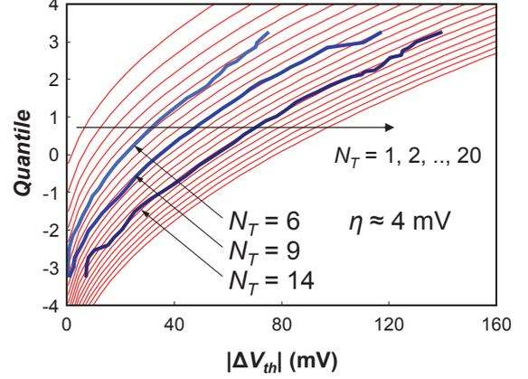
Fig. 11: Total  $\Delta V_{th}$  distribution (Eq. 2) for the average number of defects  $N_T$  from 1 to 20 (thin lines) rescaled to fit experimental distributions from Fig. 10 of Ref. [34], with the corresponding values of  $N_T$  and  $\eta$  readily extracted.
