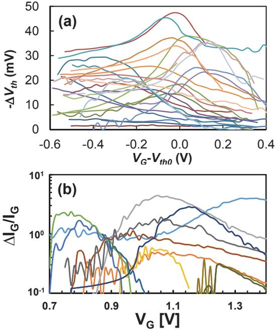
Fig. 10: (a) Different  $\Delta V_{th}(V_G)$  defect characteristics are found when measuring 30 different (but nominally identical) pFETs before and after the capture of a single hole [29]. (b) Different  $\Delta I_G(V_G)$  characteristics are found when measuring several (but nominally identical) nFETs before and after the activation of a single defect [24].
