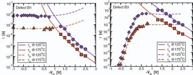
Fig. 6: Voltage and temperature dependences of  $\tau_c$  and  $\tau_e$  for two different defects. Considerable qualitative and quantitative differences between the traps are apparent [17].
