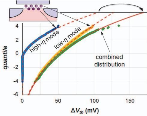
Fig. 12: Bimodal defect-centric distribution  $\Delta V_{th}$  corresponding to CHC stress: Monte Carlo and analytic fit [5,33]. The high- $\sigma$  tail of the full distribution is controlled by defects at the substrate (high  $\eta$ ; inset: solid symbols).
