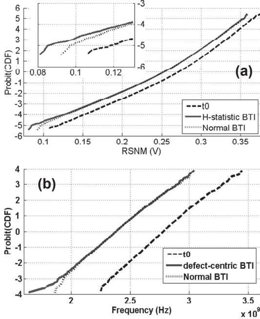
Fig. 15: (a) Probit plot of the Read Signal Noise Margin (RSNM) of 28nm technology SRAM cell for an average 50mV NBTI shift. Inset shows the discrepancy at higher quantiles. (b) Impact of binning at time-zero. Using the yield criterion of  $mean-\sigma$  on the ring oscillator frequency distributions results in a wider discrepancy between the defect-centric and Normal degradation statistics [49].
