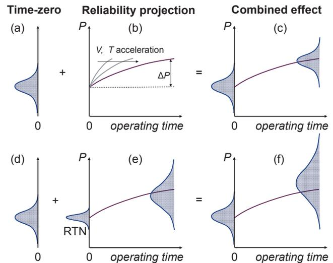
Fig. 1: A schematic representation of time-zero and time-dependent effects considered in circuit design. (a-c) Presently, time-zero variability of a device parameter  $P$  is considered together with the projection of the *mean* parameter shift  $\Delta P$  (obtained by reliability engineers through bias and temperature accelerated tests) during aging. (d-f) Time-dependent variability is also considered, in contrast to (a-c).
