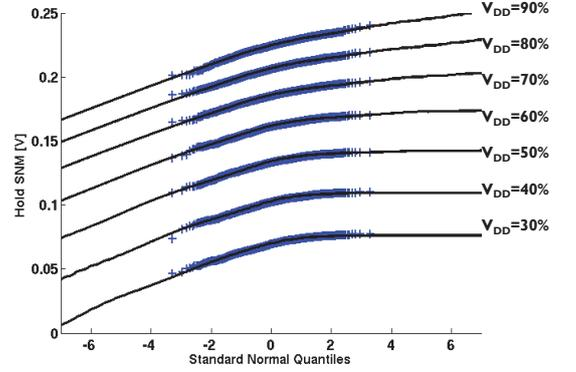
Fig. 16: Hold SNM distribution at decreasing supply voltage  $V_{DD}$ . Lines: the non-MC numerical propagation technique can predict the tails of the distribution up to  $\pm 7\sigma$ . Symbols: MC simulation added for comparison shows excellent agreement with the non-MC method [51].
