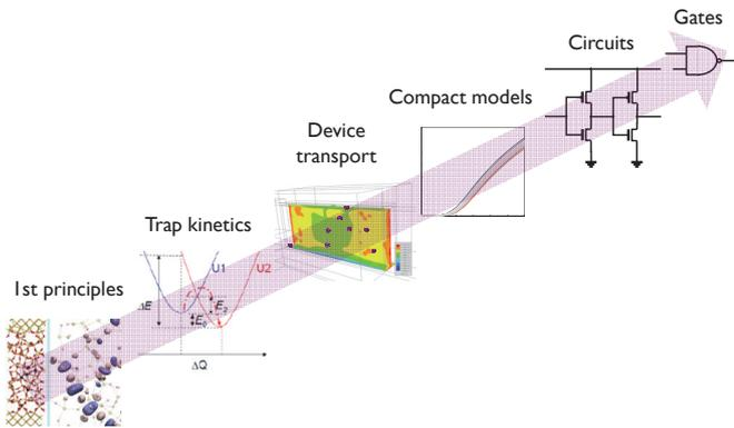
Fig. 3: Hierarchical levels of the defect-centric picture: Understanding of defect properties at the atomic level [6] can be propagated up to circuit design.
