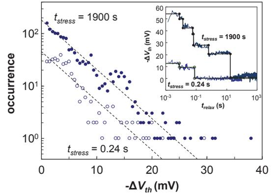
Fig. 8: Histograms of NBTI transient step heights for 72 planar Si/SiON devices show an exponential distribution. Inset: Two typical NBTI relaxation transients corresponding to the same stress times. Individual down-steps are marked with abscissas [2].
