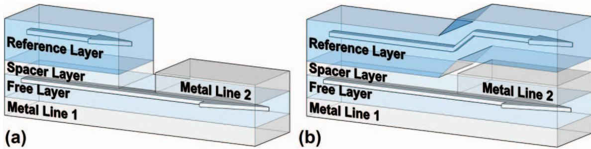
Figure 9. Schematic illustration of two memory cell structures with switching of the free layer based on the proposed "two write pulses" scheme.
