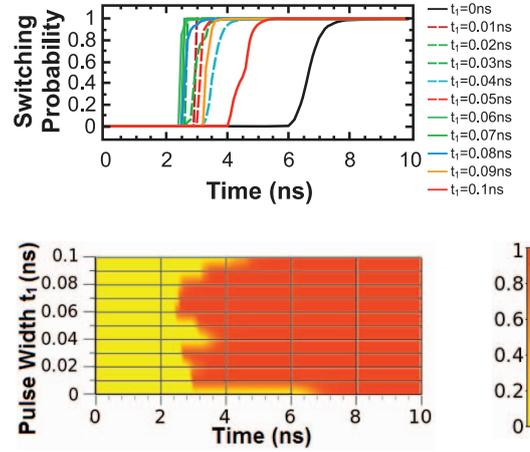
Figure 4. Switching probability for the "two write pulses" scheme as a function of the time for different values of pulse width  $t_1$ . For switching probability estimation, 250 simulations of switching were performed on each pulse width  $t_1$ .
