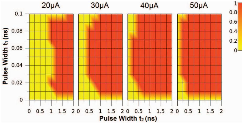
Figure 6. Schematic illustration of the dependence of the switching probability for the “two write pulses” scheme on the current and pulses width. The dependences are shown for four current values: 20μA, 30μA, 40μA, and 50μA. For switching probability estimation, 100 simulations of switching were performed on each combination of pulses’ widths.
