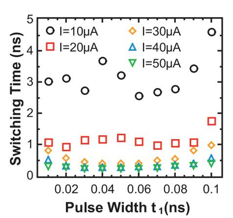
Figure 7. Switching time for the “two write pulses” scheme as a function of the pulse width  $t_1$  for five current values.
