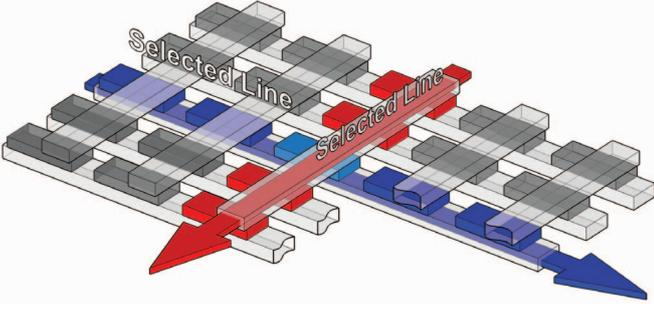
Figure 2. Schematic illustration of cross-point architecture for the switching of the soft magnetic layer by means consecutive orthogonal sub-nanosecond current pulses.
