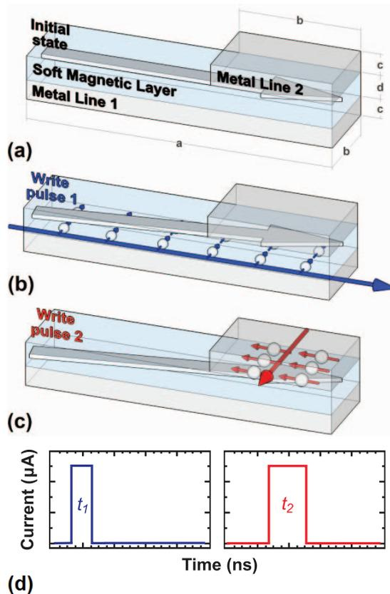
Figure 1. Schematic illustration of the proposed method of soft magnetic layer switching. In (b), (c) The direction of the charge current is shown by big arrows, the direction of the spin current is given by small arrows.
