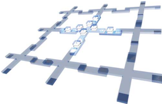
Figure 1. The spin torque majority gates (crosses) perform the computation, while the nonvolatile flip-flops (rectangles) act as shared buffers. A single STMG and three flip-flops are sufficient to realize a concatenated 1-bit full adder.
