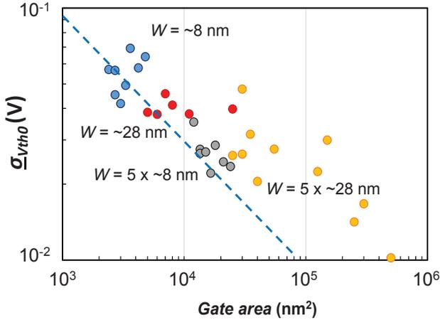
Fig. 4: Time-zero variability  $\sigma_{V_{th0}}$  of JL pFETs of varying dimensions, determined from matched pairs to compensate for across-wafer variability. The shortest devices of each  $W$  group follow approx. the expected square-root gate area dependence (dashed line) [10].
