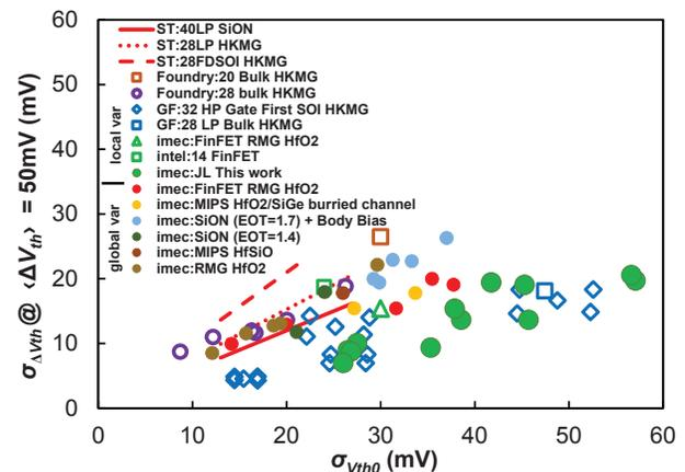
Fig. 2: Benchmark plot showing relative comparison of time-zero ( $\sigma_{V_{th0}}$ ) and time-dependent ( $\sigma_{\Delta V_{th}}$ ) variability of pFET devices for different technologies.
