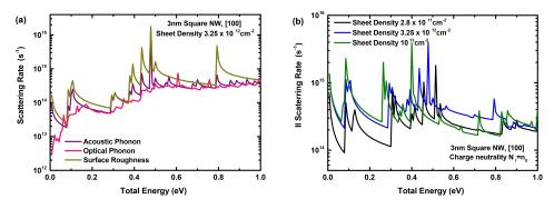
**Figure 3.** (a) The rates for acoustic and optical phonons, as well as surface roughness scattering as a function of the total energy, for a sheet density of  $3.25 \times 10^{12}$  cm<sup>-2</sup>. (b) The rates for ionized impurity scattering, as a function of the total energy and different sheet densities, assuming charge neutrality. The results are for a 3 nm diameter square nanowire structure.
