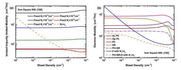
**Figure 4.** (a) Ionized impurity limited electron mobility as a function of the sheet density considering different fixed ionized impurity densities as well as charge neutrality. (b) Electron mobility as a function of the sheet density considering acoustic, optical, total phonon, surface roughness, and ionized impurity (assuming charge neutrality) scattering separately, as well as the combined mechanisms. The results are for a 3 nm diameter square nanowire structure.
