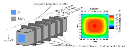
**Figure 2.** Coupling the 2D solution of the Schrödinger equation in multiple slices to a 3D Poisson solution in a structure based on a Si gate-all-around nanowire channel FET.
