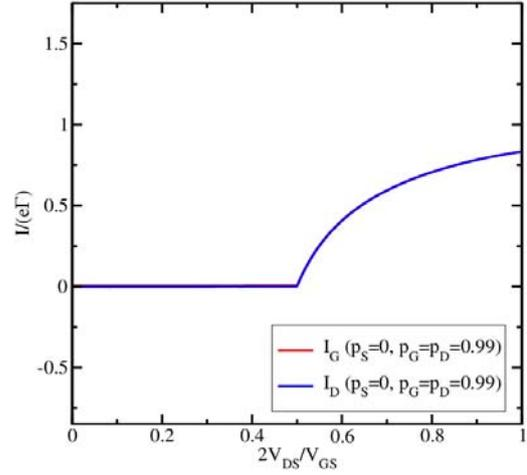
Fig.4: The currents are similar to those in Fig.3, when, in addition to the gate, the drain is ferromagnetic ( $p_G=p_D=0.99$ ).
