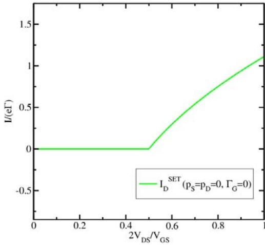
Fig.2: The SET drain current. All electrodes are normal. There is no coupling between the trap and the gate.
