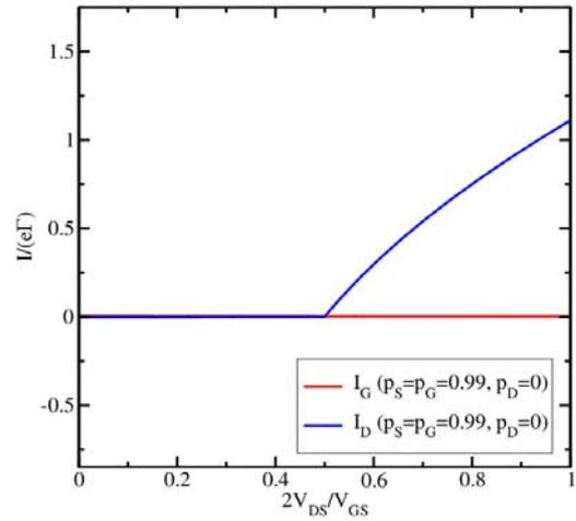
Fig.5 The gate current is suppressed when the source and the gate are ferromagnetic ( $p_s=p_G=0.99$ ).
