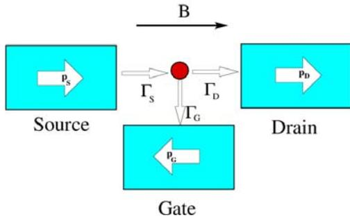
Fig.1: Schematic illustration of the device. Electron transport is caused by spin-dependent trap-assisted hopping between the ferromagnetic contacts.
