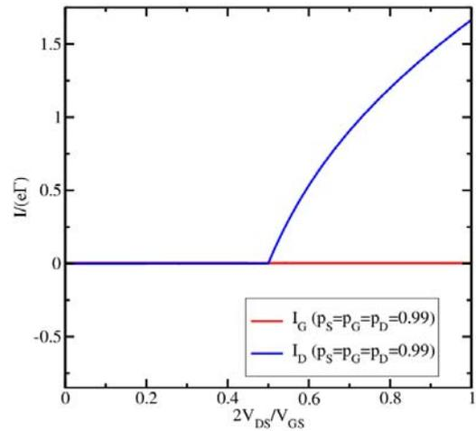
Fig.6: The drain current is the largest, while the gate current is suppressed, when all electrodes are ferromagnetic ( $p_s=p_G=p_D=0.99$ ) in the configuration shown in Fig.1.
