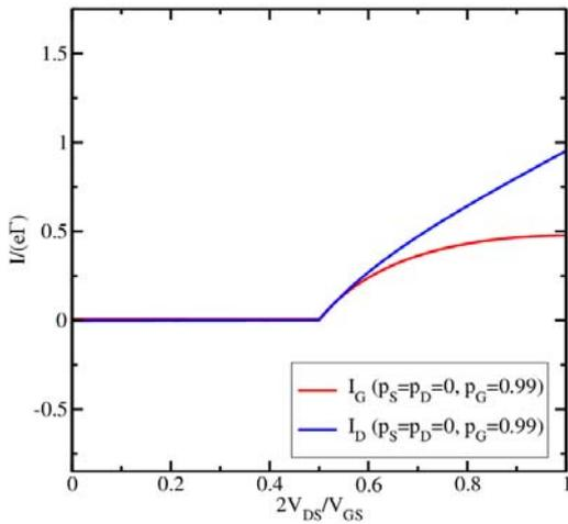
Fig.3: The drain and gate currents are suppressed, if the trap-drain junction is backward biased and the gate is ferromagnetic ( $p_G=0.99$ ). The gate current is nonzero for  $V_{DS} > V_{GS}/4$ .
