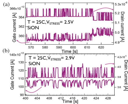
Fig 9 Both (a) positive and (b) negative  $I_D/I_G$  correlations are measured on separate SiON nFETs after stress. The negative correlation in (b) also shows signs of a second RTN path in the drain current, and is superimposed both on the low and the high state of the signal, but not visible in the gate current.
