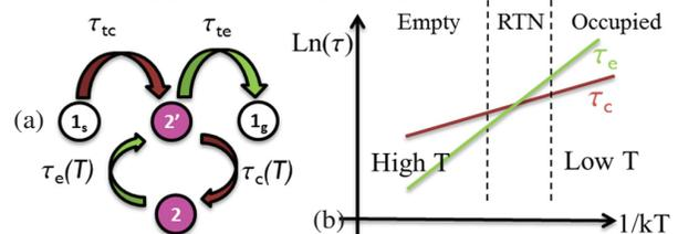
Fig 2. (a) The trap-assisted tunneling model as proposed by [9] and [10], and (b) typical temperature dependence of the time constants characterizing the transition between metastable states 2' and 2.
