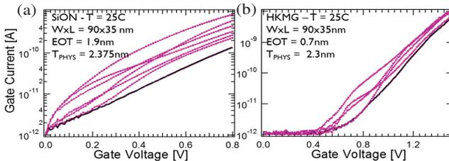
Fig. 4. Initial  $I_D V_G$ 's for different (a) SiON and (b) HKMG devices with similar physical thickness. In both cases, only a few devices show a near-perfect exponential leakage current (black lines). Other devices show a inflected  $I_D V_G$ , indicating the presence of at least one TAT-leakage path.
