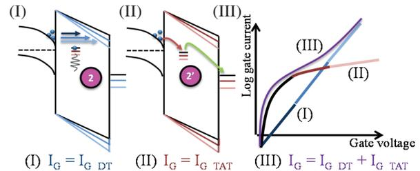
Fig 1. The schematic representation of the components of the gate leakage current. (I) A pre-existing or generated TAT-defect is charged and subsequently relaxed through multi-phonon emission. The trap cannot contribute to the gate leakage current and therefore only a direct tunneling current is measured. (II) The defect can actively contribute by trap-assisted tunneling (TAT). (III) This gate leakage path is superimposed on the direct tunneling gate leakage [9].
