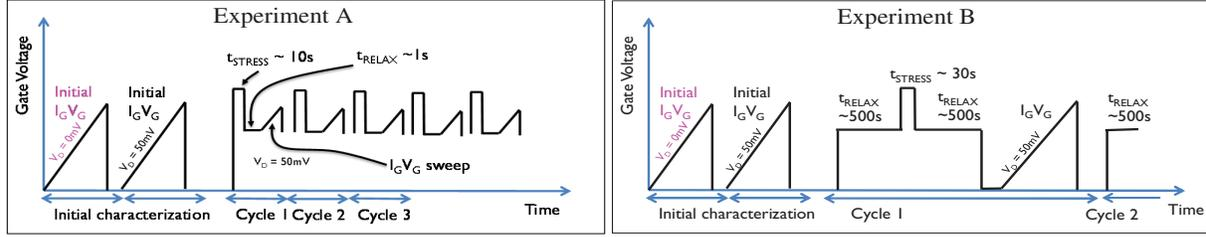
Fig. 3. Schematic illustration of the experiments performed. Experiment A provides learning about the *stress dependent evolution* of the SILC as it is focused on measuring  $I_G V_G$ s after intermittent stress cycles. The cycles are repeated 100 times. Experiment B focusses on the *time evolution and correlation* of both the gate and drain current after one short stress phase. During  $t_{RELAX}$  correlations between RTN in  $I_G$  and  $I_D$  are measured, as well as  $I_B$ .
