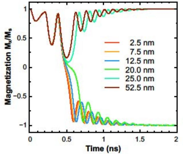
Fig. 4. The magnetization dynamics for several overlap lengths of wire NM2. Two consecutive perpendicular pulses with 30 $\mu$ A current and 200ps duration are applied.
