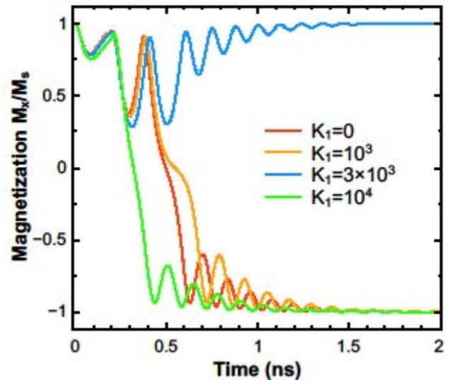
Fig. 6. Adding perpendicular magnetization if a two-pulse scheme allows to reduce the current by a factor of 6 for sub-0.5ns switching.
