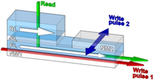
Fig. 1. Schematic of the in-plane SOT-MRAM cell. The free layer of an MTJ is grown above the heavy metal wire NM1, through which the current pulse is applied. The wire NM2 serves to conduct the perpendicular current “Write pulse 2” of the in-plane SOT-MRAM cell.
