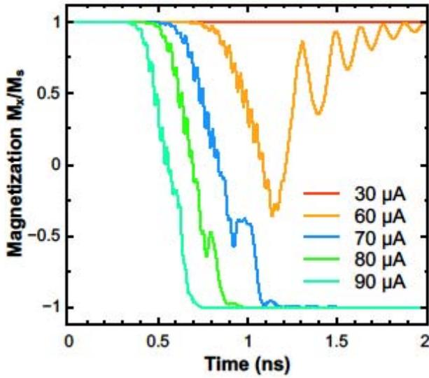
Fig. 3. Time evolution of the magnetization for several values of the current through wire NM2 with the width 12.5nm. The current through wire NM1 is zero.
