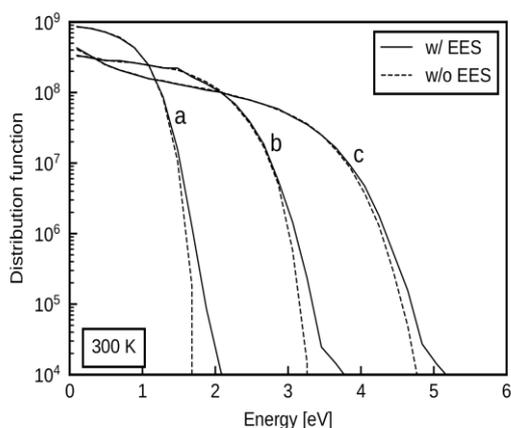
Fig.4: Enhancement of the high energy tail due to EES. The potential profile and three lateral positions reported in [2] have been used.
