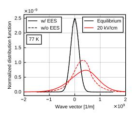
Fig. 1 Momentum distribution functions at equilibrium and at 20 kV/cm, lattice temperature 77 K.
