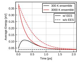
Fig. 3 Relaxation of the mean energy is affected by EES. The initial two-particle distribution function assumed consists of a hot ensemble at 3000K and a cold ensemble at 300K.
