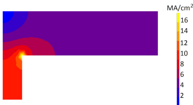
FIG. 12. (a) Current density distribution map in the cathode area shown strong crowding at the via-line conjunction.
