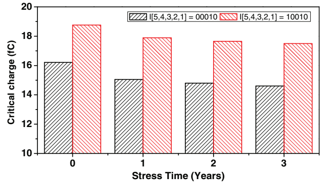
FIGURE 11 Critical charge at the sensitive node (S) of the c17 circuit for two worst-case input combinations with the different stress time
