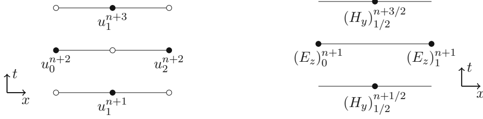
Figure 9: Leap-frog scheme (left) and Yee's scheme (right) in 1D. The labeled nodes are related to each other in an update step through centered finite differences in space and time around the central point. White nodes do not participate in the update of labeled nodes and thus the leap-frog scheme effectively does two independent FDTD-like simulations on one grid.
