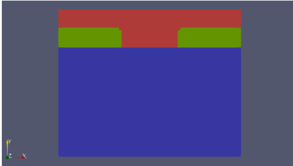
Figure 4: The geometry for the dopant in-diffusion example. The semiconductor substrate at the bottom (blue) is covered with a mask layer (green) with a hole in the middle, where it is exposed to the surrounding fluid or gas (red) with a certain material concentration.
