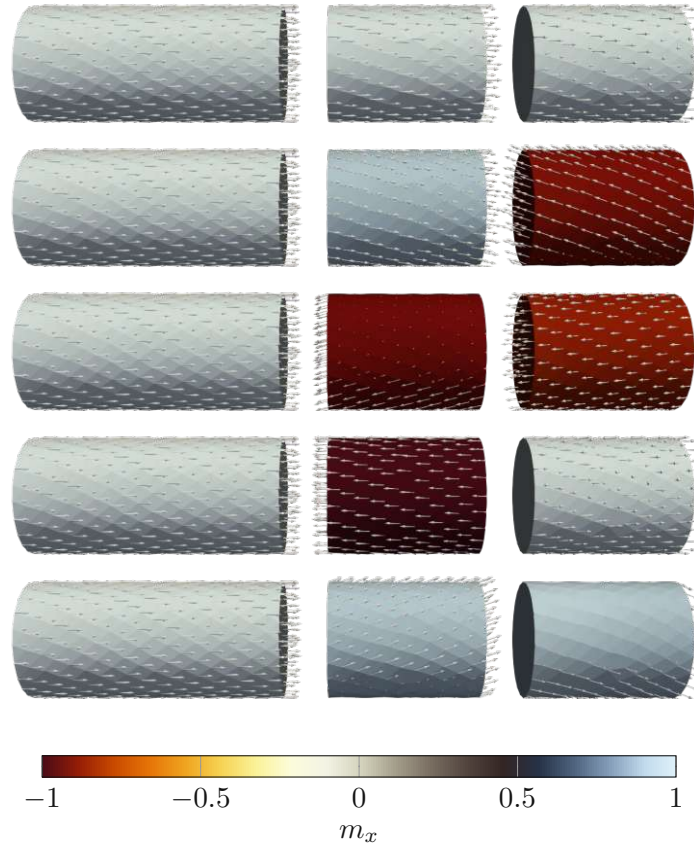
Figure 7.16: Cyclic switching visualization during P→AP transition: three-dimensional magnetization snapshots at five characteristic stages (i)–(vi) of the FL reversal cycle, colored by the m_x magnetization component. Based on [199].
