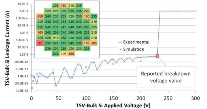
Fig. 7. TSV bulk Si leakage current as a function of applied voltage. Inset: TSV breakdown voltage [V] (Cassidy et al. [9]).
