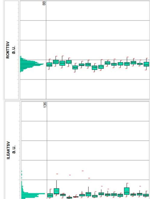
Fig. 10. Stability of wafer acceptance test parameters, such as TSV resistance (top) and TSV leakage (bottom), over multiple manufacturing lots.
