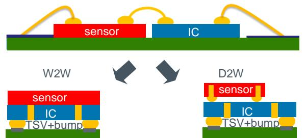
Fig. 2. Form factor reduction for sensor and IC system in a package by replacing wirebonds with TSV and bumps. Integration by W2W bonding for matched sensor and IC die sizes (bottom left) and D2W stacking, if the IC die size is larger than sensor die size (bottom right).
