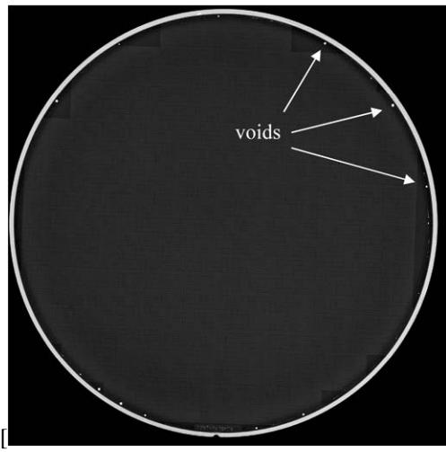
Fig. 8. SAM image of a direct bonded sensor and IC wafer pair. White spots near the wafer edge are voids (Kraft et al. [8]).
