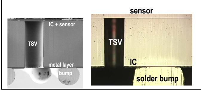
Fig. 3. SEM X-section of an active silicon interposer from Fig.1 (left) and a 3D integrated (photo-) sensor and integrated circuit from Fig.2 (right).
