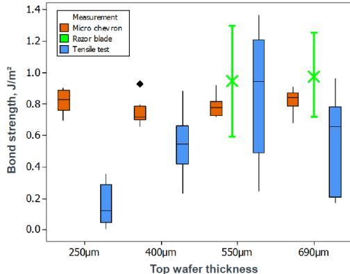
Fig. 9. Comparison of the accuracy of prior destructive bond-strength measurement methods with the Micro-Chevron test (Siegert et al. [13]).
