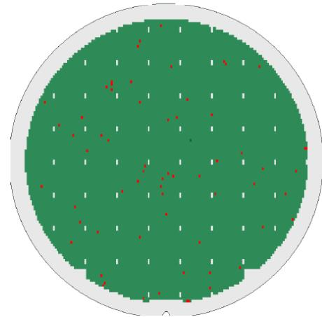
Fig. 11. Wafer map showing a typical production test result for the active interposer with SoC integrated sensor and IC as well as TSV, backside redistribution layer, and bumps as shown in Fig.2 (left). Red dots show failing sites. Overall yield is > 99.5% for a chip size of ~2mm<sup>2</sup>.
