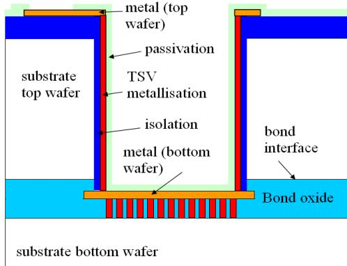
Fig. 4. Schematic cross-section of an open TSV (Kraft et al. [8]).
