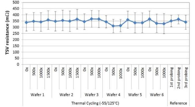
Fig. 6. TSV resistance as a function of thermal cycles versus reference (Cassidy et al. [9]).
