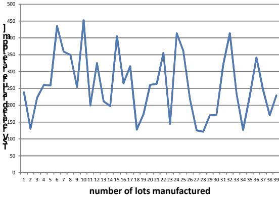
Fig. 12. Typical TSV related failure rate for mass production.
