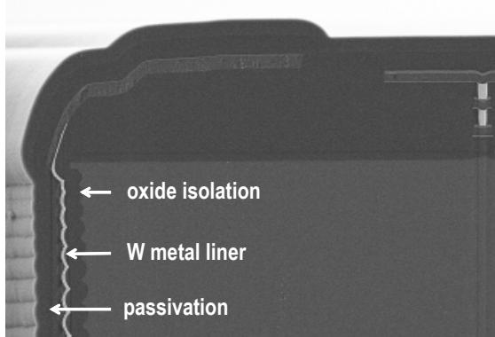
Fig. 5. Top edge cross-section of an open TSV.
