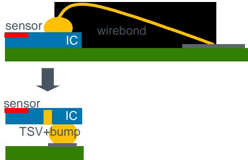
Fig. 1. Form factor reduction for SoC integrated sensor by replacing wirebonds with TSV and bumps.
