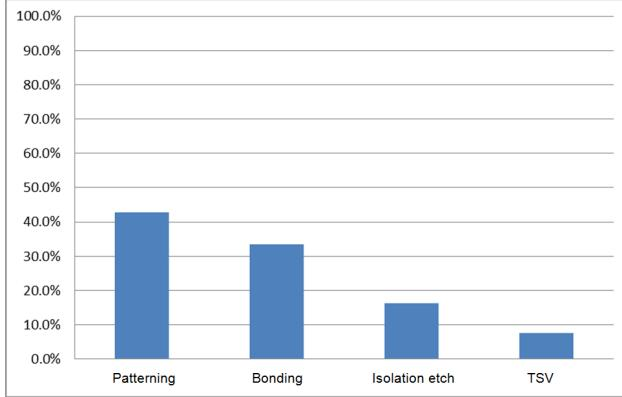
Fig. 13. Yield Pareto distribution for the TSV related failures for the IC with a 3D integrated photodiode shown in Fig.2 (right). The chip size is ~100mm<sup>2</sup>.
