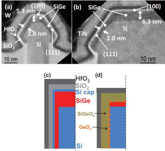
Fig. 2. TEM micrographs of SiGe cladding fins with Si cap, nominal fin width (a) 20nm, (b) 130nm. Notice the thinner SiGe on the sidewalls. (c) Idealized gate stack sketch for SiGe cladding finFET w/ and (d) w/o Si cap. In the latter case, the direct oxidation of the SiGe channel might induce the formation of detrimental Ge suboxides, limited by the relatively low Ge fraction in the SiGe channel.
