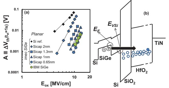
Fig. 1. (a) NBTI-induced  $\Delta V_{th}$  in planar Si reference and SiGe channel pMOS [7]. Both a reduced NBTI and a steeper voltage acceleration have been observed in SiGe (imec and IBM [8], [9] data), and ascribed to (b) a reduced interaction with oxide defects thanks to a favorable energy alignment [7].
