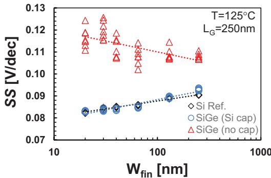
Fig. 3. Subthreshold swing vs.  $W_{fin}$ . Si cap passivation yields optimal, Si-like interface quality; note the improved electrostatics for narrowing  $W_{fin}$ . Direct oxidation of SiGe (no cap) yields degraded interface due to  $GeO_x$  formation, particularly on sidewalls (narrow  $W_{fin}$ ) where the thinner SiGe might be fully oxidized.
