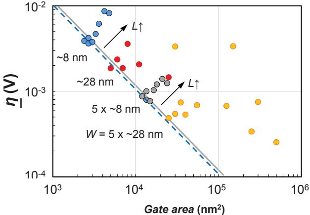
Fig. 5: Time-dependent variability of JL pFETs, extracted from matched pairs [12] and expressed via the mean impact of a single trap  $\eta$ . The shortest devices follow reciprocal area dependence (dashed line), similar to pFinFET devices (gray solid line) [6]. Longer devices in each group show increased variability (arrows), likely due to narrowing of wires caused by processing.
