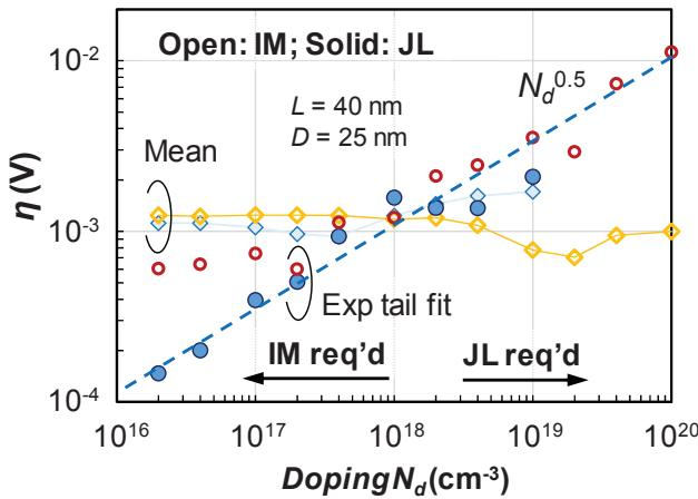
Fig. 12: Simulated impact per single trap  $\eta$ . Exp-tail-fit  $\eta$ , extracted as shown in Fig. 10, follows approx.  $N_d^{0.5}$  dependence on doping (dashed line). Required doping trends for IM and JL devices are indicated by arrows.
