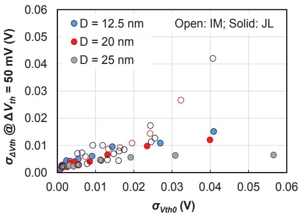
Fig. 13: IM and JL pFETs simulation results (time-zero: Fig. 5; time-dependent: Figs. 6-8) arranged into the benchmark plot (Fig. 2). The relatively low  $\sigma_{\Delta Vth}$  of JL FETs observed experimentally (Fig. 2) is reproduced. (In this plot only, simulation results of different NW dimensions are shown.)
