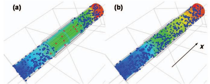
Fig. 1: Illustration of (a) Inversion Mode (IM), and (b) Junctionless (JL) GAA NW FET devices (spheres: dopants). High current and hence high carrier concentration are achieved by high doping of source and drain regions. By the nature of the JL device, this implies high doping of its body as well.
