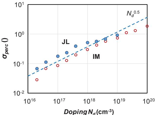
Fig. 9: The scale parameter  $\sigma_{perc}$ , controlling the width of the log-normal  $\Delta v_{th,RDD} / \Delta v_{th,CONT}$  distributions in Fig. 8, increases with  $N_d^{0.5}$  for both IM and JL GAA NW pFETs.
