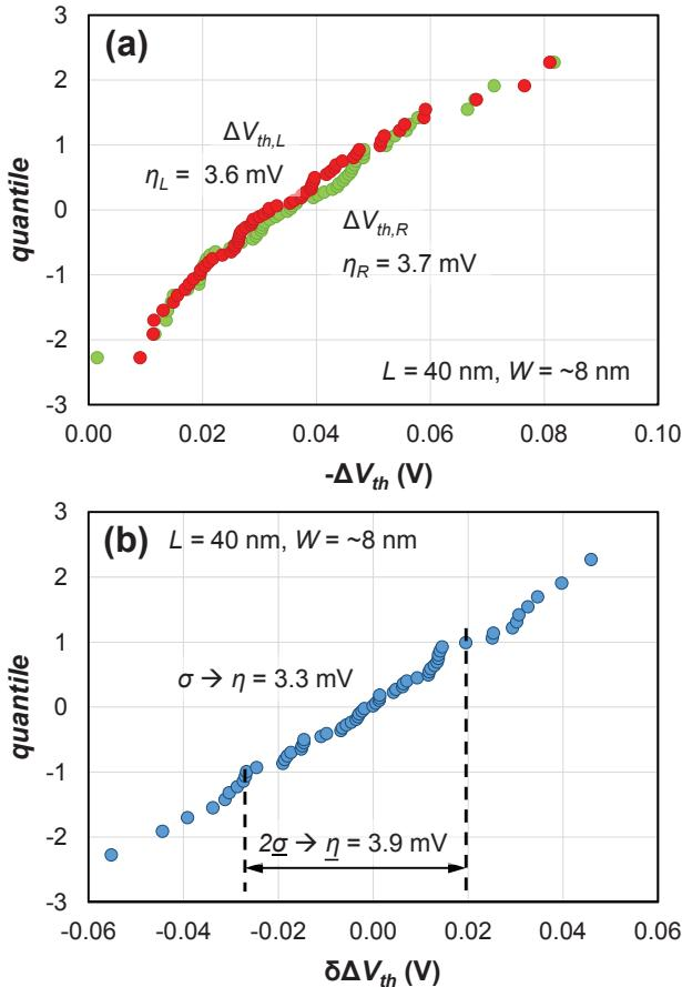
Fig. 3: (a) Well-behaving (i.e., without outliers) “defect-centric” distributions for “Left” and “Right” devices with the  $\eta$  values extracted using Eq. 3 indicated. (b) The distribution of  $\delta\Delta V_{th}$  calculated from the corresponding values  $\Delta V_{th,L}$  and  $\Delta V_{th,R}$  of each matched pair taken from (a). The distribution is approximately Normal. The “robust” value (underlined) correctly reproduces the standardly-obtained value of  $\eta$ .
