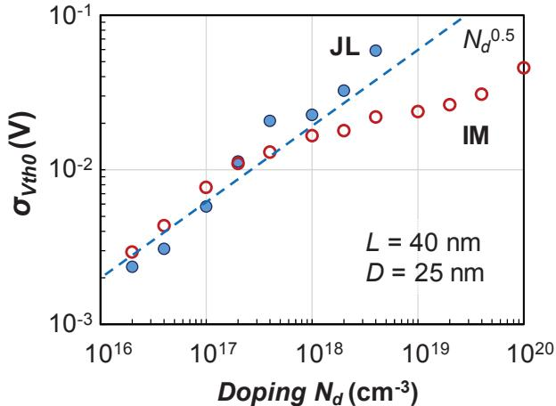
Fig. 11: Simulation of simplified IM and JL GAA NW pFETs shows the time-zero variability  $\sigma_{Vth0}$  of both types of devices is broadly identical and follows approx. square-root dependence (dashed line) at lower doping levels.
