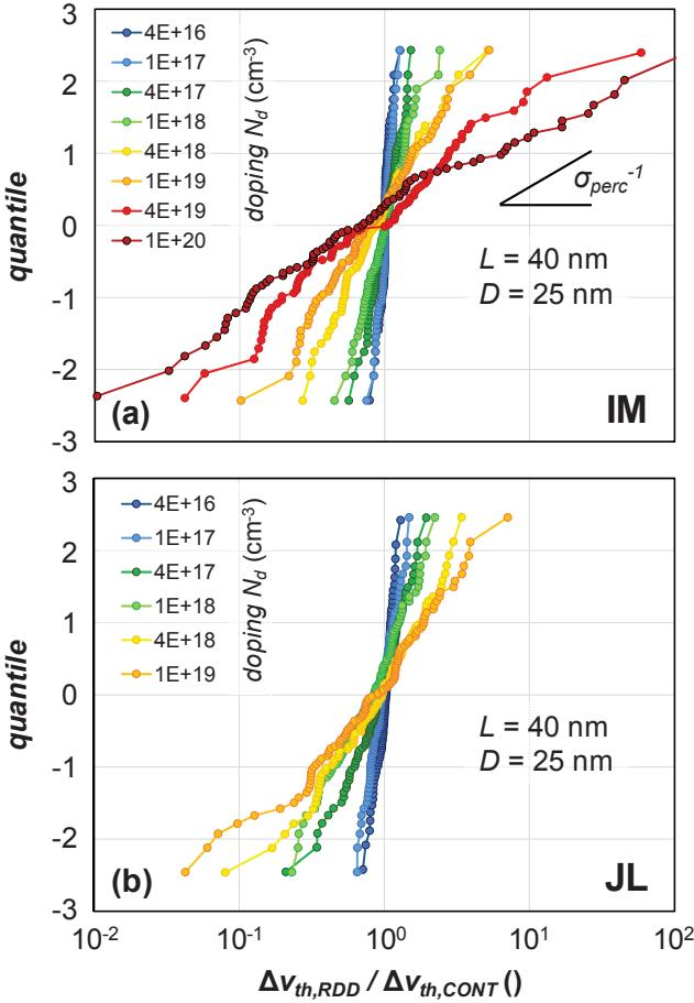
Fig. 8: The ratio of  $\Delta v_{th,RDD} / \Delta v_{th,CONT}$  constitutes the added impact of RDD to the device electrostatics (i.e.,  $\Delta v_{th,CONT}$ , cf. Fig. 7). The distributions of this ratio can be acceptably described with a log-normal with parameter  $\sigma_{perc}$  for both (a) IM and (b) JL GAA NW pFETs, for a wide range of doping levels. Note: IM distributions are simulated to higher doping levels, resulting in wider distributions than those of the JL devices.
