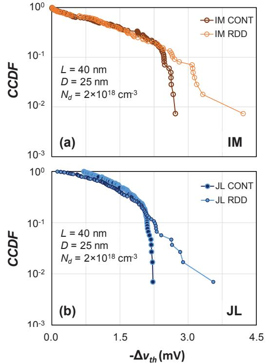
Fig. 7: Simulated  $\Delta v_{th}$  profiles from Fig. 6 are sorted into Complementary CDF (CCDF) plots for (a) IM and (b) JL GAA NW pFETs. RDD adds an approximately exponential tail to the CONT distributions.
