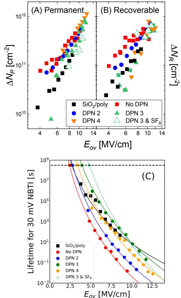
**Figure 5.** Universal Model fit results show (A)  $\Delta N_P$  and (B)  $\Delta N_R$  changes with  $E_{ov}$  as a function of DPN intensity, while (C) shows the estimated lifetime for 30 mV plotted against the effective field,  $E_{ov}$  (i.e.  $V_{ov}/EOT$ ) for the samples. An optimum in NBTI robustness with DPN3, which is further enhanced by F incorporation is shown.
