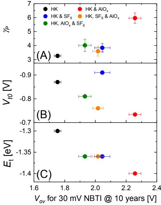
**Figure 14.**  $V_{ov}$  for 30 mV NBTI degradation observed on  $\text{AlO}_x / \text{SF}_6$  incorporation of  $\text{TaN/TiN}$ -gate stacks correlates with (A) accessibility to near-interface permanent defect band,  $\gamma_p$ , from Universal Model fitting, (B) initial  $V_t$ , and (C) donor-band defect trap energy level, with respect to  $E_{F_i}$  silicon, derived from Comphy
