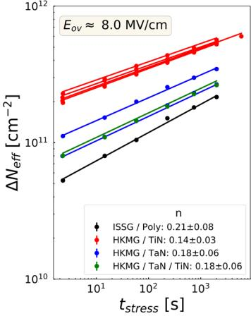
**Figure 8.** Defect generation kinetics as a function of gate electrode, showing higher  $\Delta N_{\text{eff}}$  and lower time exponent for TiN based stacks, than TaN-based or poly/SiO<sub>2</sub> reference.
