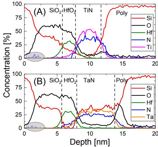
**Figure 6.** EDS signal from TEM measurements shows higher N content in  $\text{SiO}_2$  for (A) TiN than (B) TaN-gated HKMG stacks.
