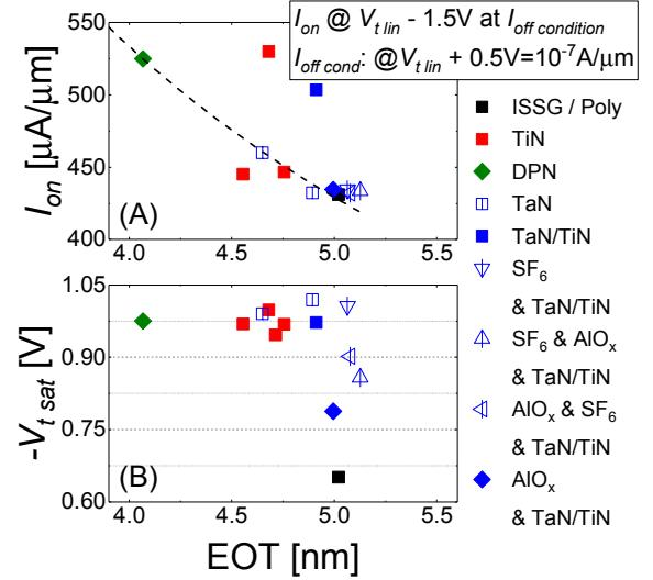
**Figure 10.** (A)  $I_{\text{on}}$  and (B)  $V_t$ -EOT trends for novel stacks HKMG explored, showing negligible impact on device performance, and strong  $V_t$  reduction on AlO<sub>x</sub> incorporation.
