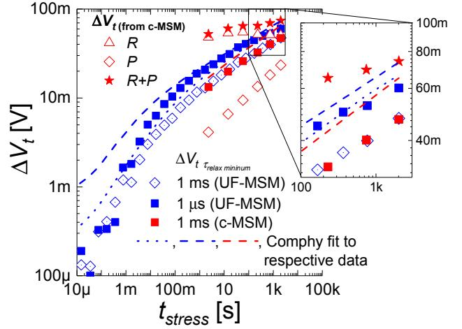
**Figure 2.** Defect kinetics revealed by conventional and Ultra-Fast-MSM (c and UF, respectively) are comparable for 1 ms  $t_{\text{relax minimum}}$ .  $\Delta V_t$  from Universal Model Fitting (to which Comphy fits converge) exceeds  $\Delta V_t \tau_{\text{relax}} \geq 1\mu\text{s}$ , suggesting fast-trap (<1 ms) contribution detected by Universal model [6] fits to c-MSM data.
