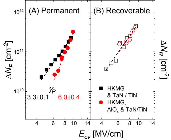
**Figure 13.** Impact of AlO<sub>x</sub> cap on (A)  $\Delta N_P$  and (B)  $\Delta N_R$  for TaN/TiN-gated samples is limited to the permanent defect contribution, which shows lower density and higher bias dependence.
