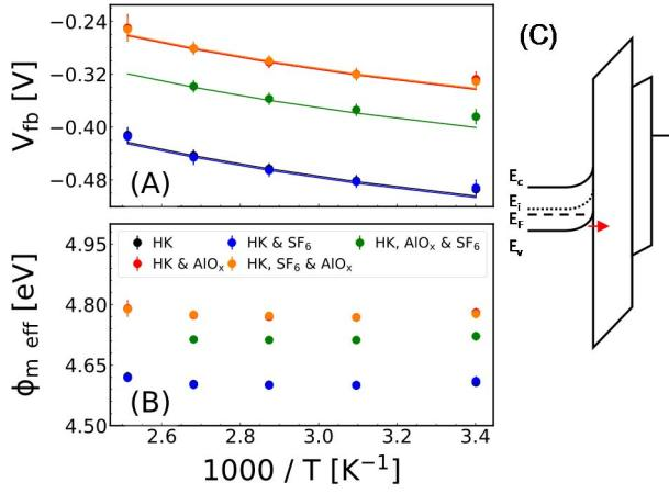
**Figure 11.** Results from Capacitance-Voltage measurements show (A) measured (symbol) and fitted (solid line) flat band voltage,  $V_{fb}$ , and (B) effective work-function,  $\phi_{m\ eff}$ , as a function of measurement temperature, while (C) shows the band alignment corresponding to the accumulation of the  $p$ -Si substrate.
