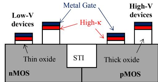
**Figure 1.** Schematic diagram of varying oxide thickness on devices in the periphery of memory devices, enabling fabrication of varying-V<sub>dd</sub> devices utilising a single high- $\kappa$ /Metal gate process, albeit on multiple oxide thicknesses.
