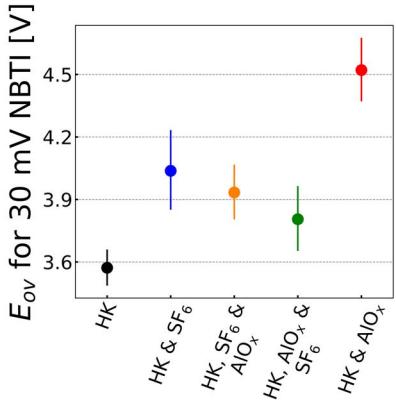
**Figure 12.**  $E_{ov}$  for 10-year NBTI lifetime at 30 mV degradation for TaN/TiN-electrode stacks examined, showing a significant increase on AlO<sub>x</sub> incorporation into the pFET devices. Intermediate values are attained after SF<sub>6</sub>, with or without AlO<sub>x</sub>.
