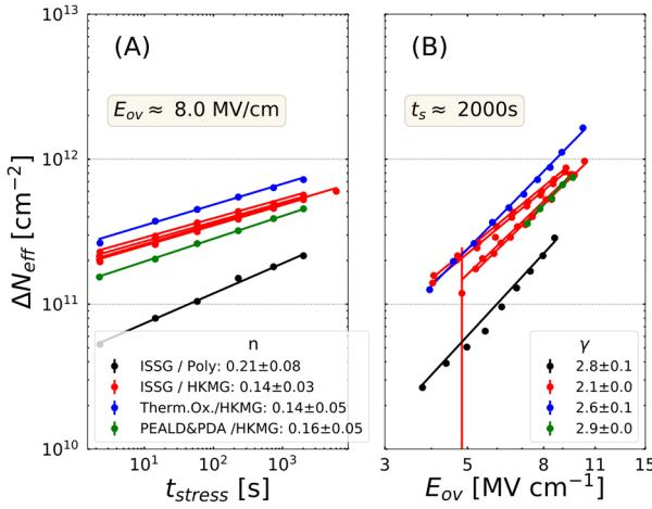
**Figure 3.** Defect generation (A) kinetics and (B) bias dependence for Si/SiO<sub>2</sub>/HK/MG stacks, where the SiO<sub>2</sub> fabrication method was varied. Similar characteristics for all SiO<sub>2</sub> oxidation methods are shown and have higher defectivity than the poly/SiO<sub>2</sub> reference.
