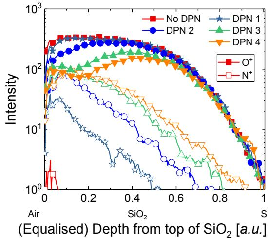
**Figure 4.** N<sup>+</sup> and O<sup>+</sup> profiles from ToF-SIMS, in SiO<sub>2</sub> layers subjected to DPN steps of varying intensity, show the modification of the interlayer as a function of the DPN step applied. Profiles were equalised to ensure Si signals overlap, with the Si/SiO<sub>2</sub> interface located between 0.6 and 0.7 x-axis
