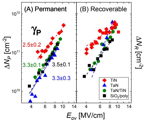
**Figure 7.** Permanent and Recoverable defect densities derived from Universal Model fitting of NBTI data for the gate-electrode options explored, reveal that TiN-gated stacks results in higher (A)  $\Delta N_P$  and (B)  $\Delta N_R$ , together with higher bias dependence for both defect types.
