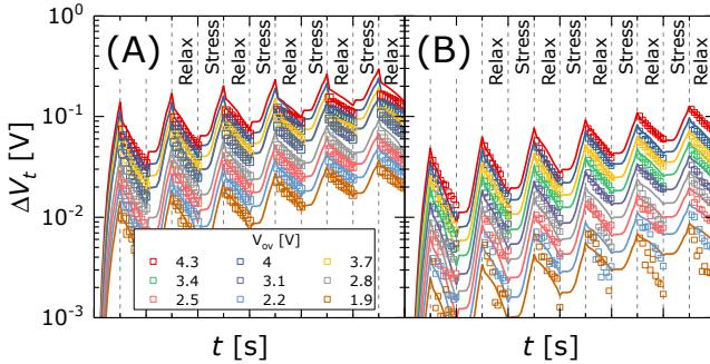
**Figure 9.** Measured  $\Delta V_t$ -t data at varying  $V_{ov}$  (symbols), during consecutive stress (incrementing from ~2 to ~1000s) and relax (1ms-10s) cycles for (A) TiN and (B) TaN-gated stacks. Solid lines are Comphy fits of measured dataset. Each stress and relax step are plotted on their own individual log scale.
